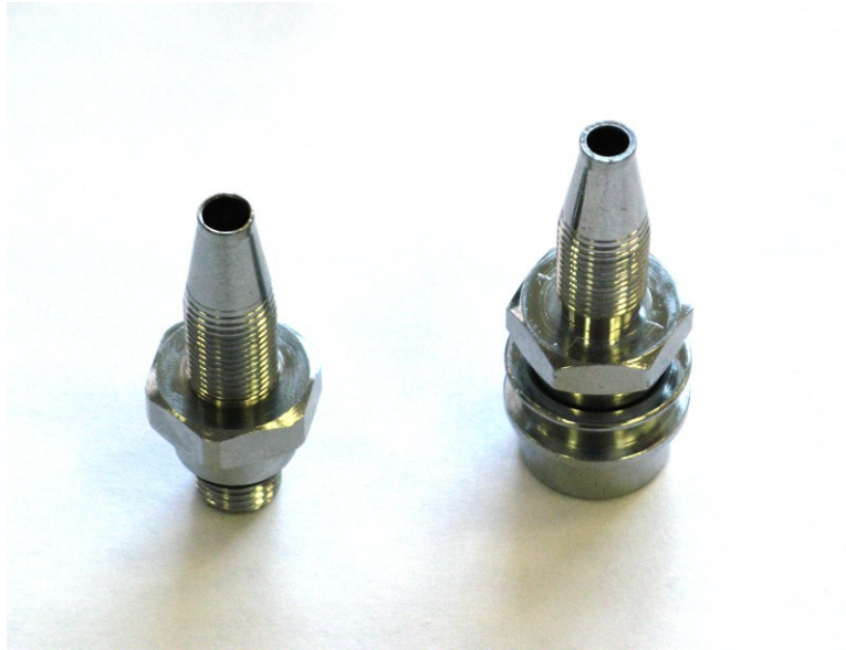
Fig 3-4-1: “Crimp and reusable fittings compared, inner core. It is essential that the end of the fitting is rounded to prevent the fitting cutting into the inner hose. All incoming material shall be inspected to ensure the fitting end is rounded, free of burrs and oxygen compatible grease shall be used on the end of the fitting when it is inserted into the hose to avoid it cutting the hose. Both the above fittings should fail the inspection for no sharp edges.
