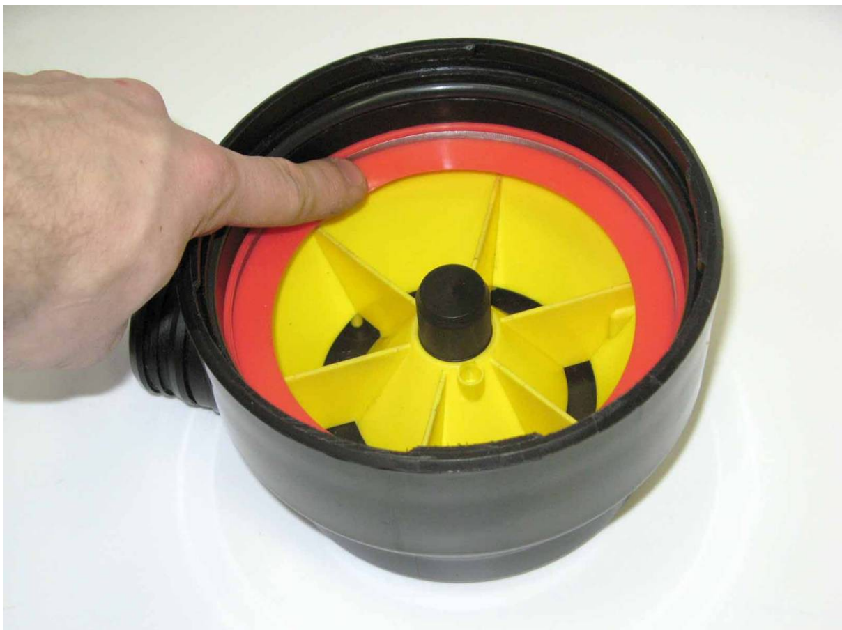
Fig 4-36: EAC seal moulded in red, contrasts well with both black and yellow flow cones, allowing the diver to inspect the seal easily each time and EAC is fitted.
