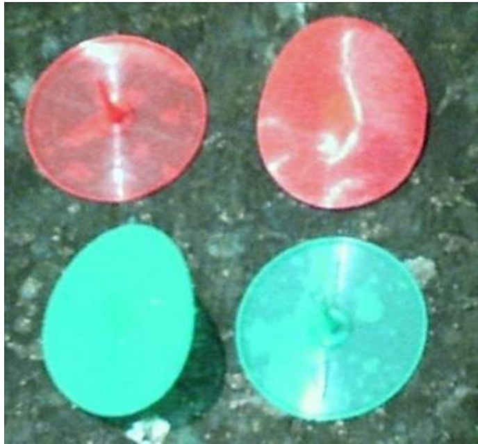
Fig 4-13: Flat flapper valves produced using the injection mould tooling, showing the colour coding matching the hose caps. The top left valve and bottom right valve has sealed to the smooth granite surface under its own weight.
