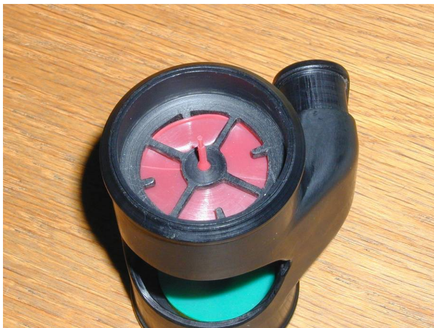
Fig 4-15: Example of flapper valve failure with half finger alternatives (rejected). A plain DSV was used for these tests.
