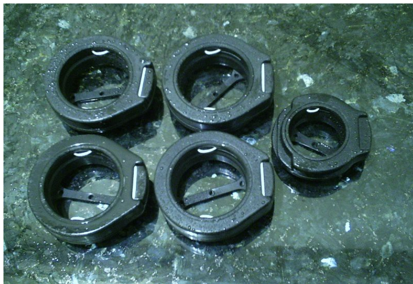
Fig 4-5: Four of the first generation Press-Click connectors used for the project with a Draeger P Port for comparison. In the review of the project, it was concluded that this solution does not meet the safety requirement: two distinct actions are required. The SCR is pressurised during ascent, so the pull action happens automatically due to the pressure
