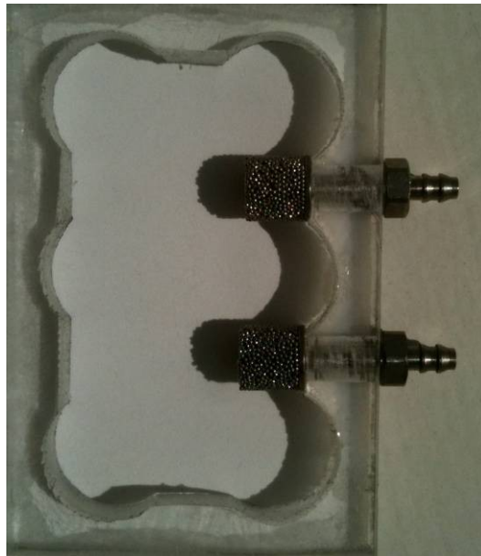
Figure 4-2: Outlet filter: the injector system (each rebreather) supplies gas into a connection shown on the right above. The gas passes through a sintered filter to disperse the gas flow, and then out of a hydrophobic membrane (bright white in the above image). The membrane has a large area, secured to a frame.
