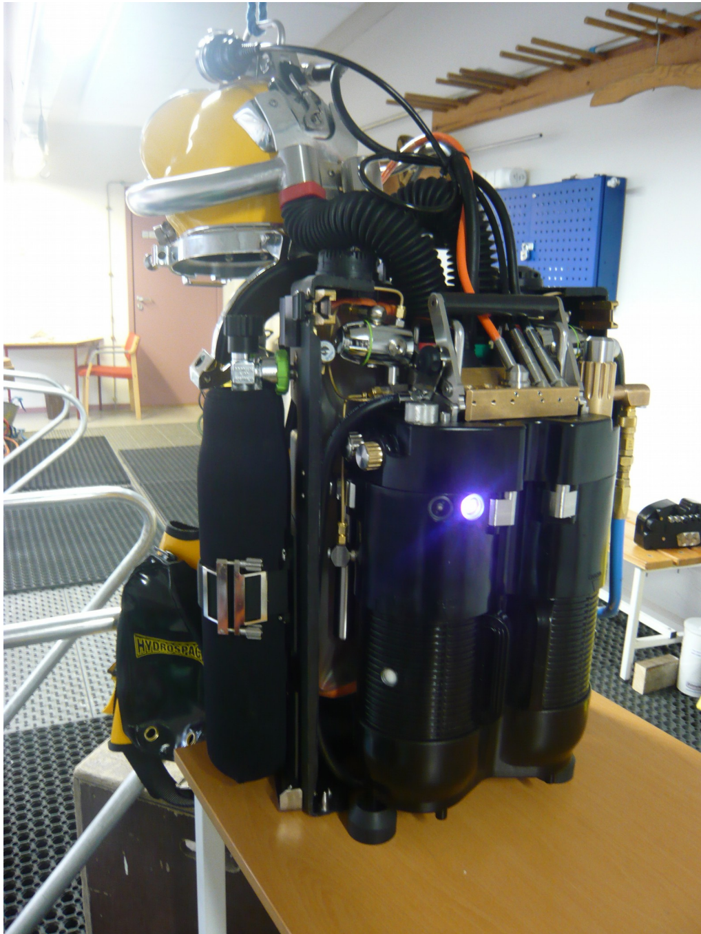
Fig 4-33: Commercial diving scrubber canister assembly showing viewing ports and buddy status lights.
