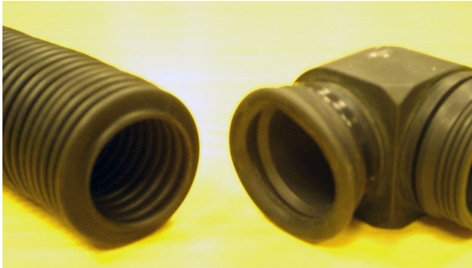
Fig 4-9: Hose failure on a 50kg load on a sample of the thermal re-formed hose. Note hose is still attached to port: the test was carried from port to mouthpiece. The cable clamps have not yielded and the creep is less than 1mm. Tests were carried out with both plastic clamps and stainless steel Jubilee clip clamps (that are used to attach the hose in production), in case a diver replaces the Jubilee clip with a cable tie in the field. Microscopic examination of the failure shows it to start at the point where the forming tool has grabbed the hose during its manufacturing process: there is a 0.3mm deep cut on every ring of the hose where this failure can start. The hose material was subsequently improved and the thickness increased: the new hose withstands a 100kg pull.
