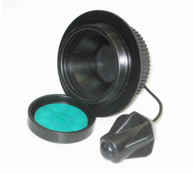
Fig 4-7: Original water dumps using one way valve and dump valve. Short toggle shaped to avoid snagging the dump. The cord is a Bowden cable, in May 2010, improved further by shortenng the cable to remove all slack in June 2010.
