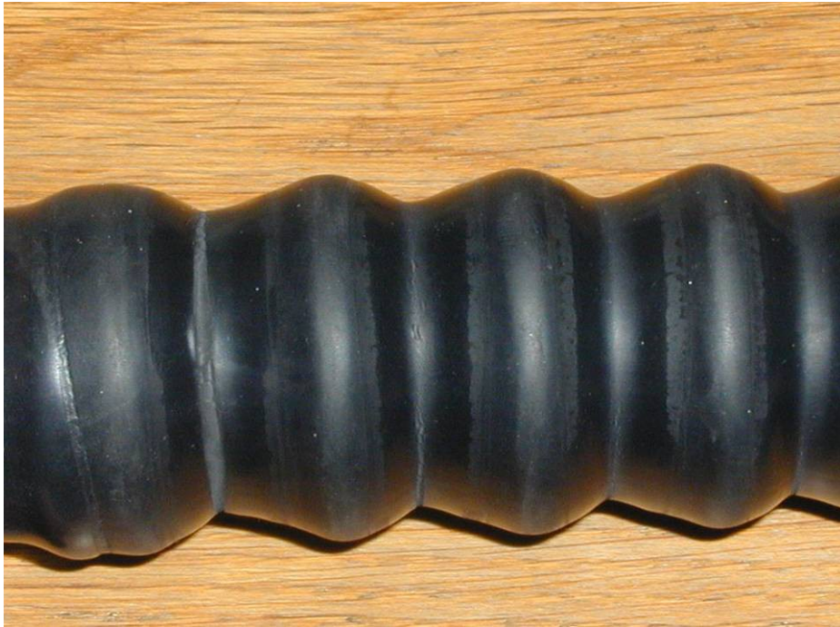
Fig 4-10: Hose under tension showing cracks caused by forming tool during manufacture, from which failures extend around the hose. Manufacturer agreed to address this by much more frequent cleaning of the forming tool than for non-critical applications. New hoses withstand a 100kg pull test.
