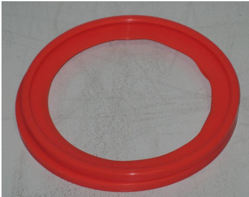
Fig 4-35: EAC seal after three days of immersion in silicone oil, showing swelling but otherwise still functional. The seal is tolerant of all other common chemicals, and of strong bases (caustic compounds).
