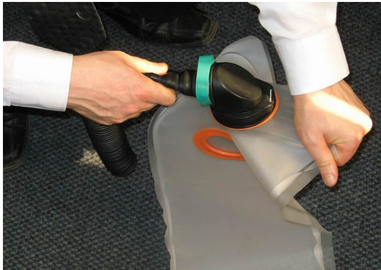
Fig 4-32: Test of counterlung port reinforcement and mating with maximum force to pull the hose from the bare counterlung using thinner counterlung TPU to increase the stretch: the production TPU is 600 micron thick and not easily stretched. Even under these conditions hose was retained. The example above uses the thinnest counterlung material. The above test was configured specifically using counterlung material that would manifest the failure if the failure mode existed. This test was repeated with a 50kg and 100kg weight, without any failure of the hose clamp, hose, port or port from the counterlung. Test indicates that the reinforcement ring is effective at achieving its designed function, namely to prevent the failure where the port pulls free of the counterlung.
