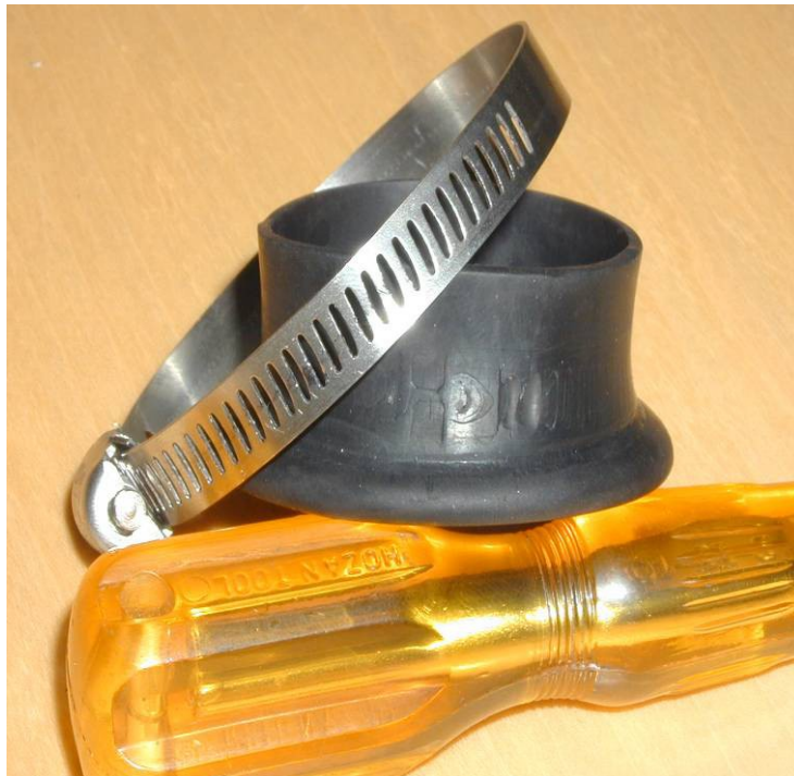
Fig 4-11: Hose with jubilee clip, after tensioning the clip until the grub screw failed, then tensioning the hose until the hose failed. Hose failure point is at the same point observed in the tests reported in the previous section. The hose is attached using a Jubilee clip identical to the one shown, at both ends, in all configurations of the rebreathers.
