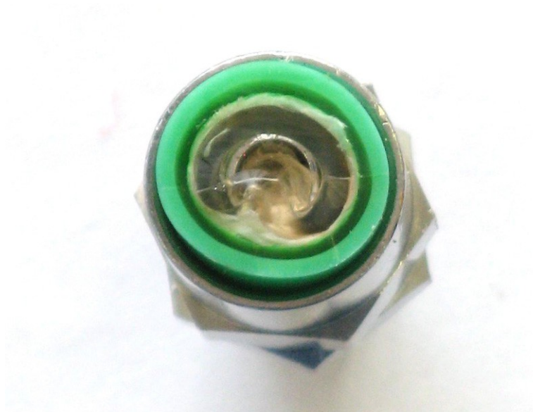
Fig 3-4-1: Section through hose that fails with a test pressure of 90 bar, showing how the reusable inner fitting has cut through the inner hose allowing gas to leak into the sheath.
