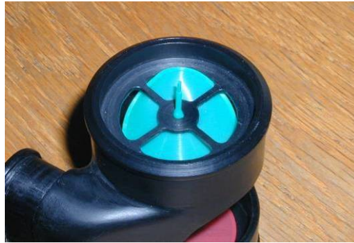
Fig 4-16: Example of flapper failure with four finger alternative. The valve does correct itself immediately when breathed, but as four fingers can leak, five fingers was regarded as the borderline case and the design was set to the web with six fingers. The face of the web seen here is being moulded, with projections to prevent the flapper being inserted on the top surface, and the web colour matching the flapper component.
