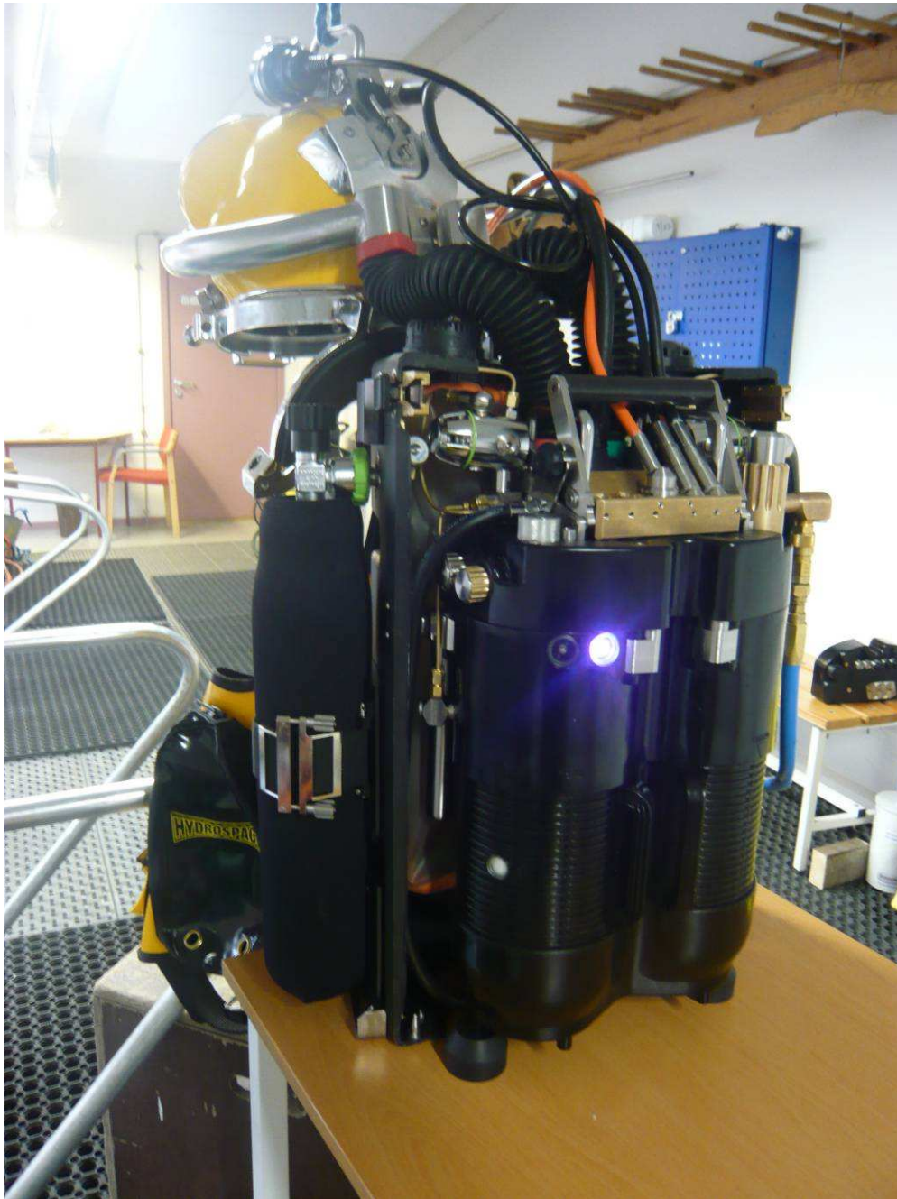
Figure 9-1. DL DRB Rebreather for Commercial Diving, shown here operating, with back cover removed. Counterlungs are in the same position as for the single scrubber configuration, and of the same construction, but the scrubber fixed body is further out from the diver: it is connected by a rigid manifold. The corrugated hose is the same, but there is an additional run of stainless steel tube around the helmet, and a gas heater.
