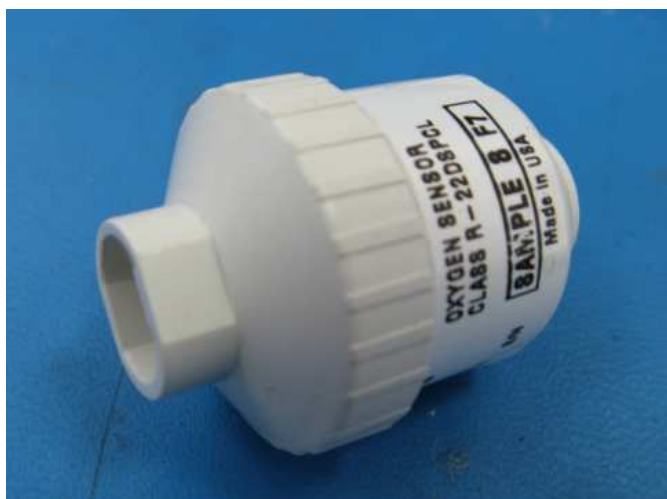
Figure 20.1 -Example of sensor marking. Sensor 8 had an output mean of 9.743 mV in air at a mean temperature of 24.62C. Date code is F7 rather than JULY 2007 but otherwise is clear.
