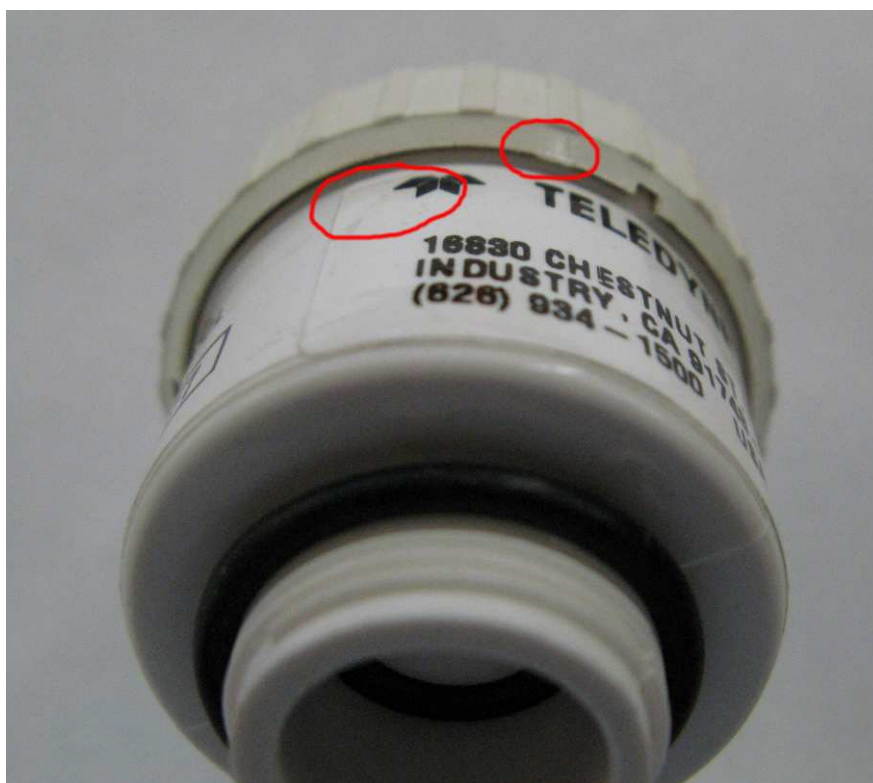
Figure 20.7- Electrolyte drops marked in red on the body of Sample 2
