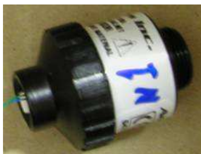
Fig 19.1-1. Sensor marking. Sensor 1 had an output mean of 11.94 mV in air at a mean temperature of 24.91 C. All others were in the range 11.85 to 12.0mV under similar conditions.
