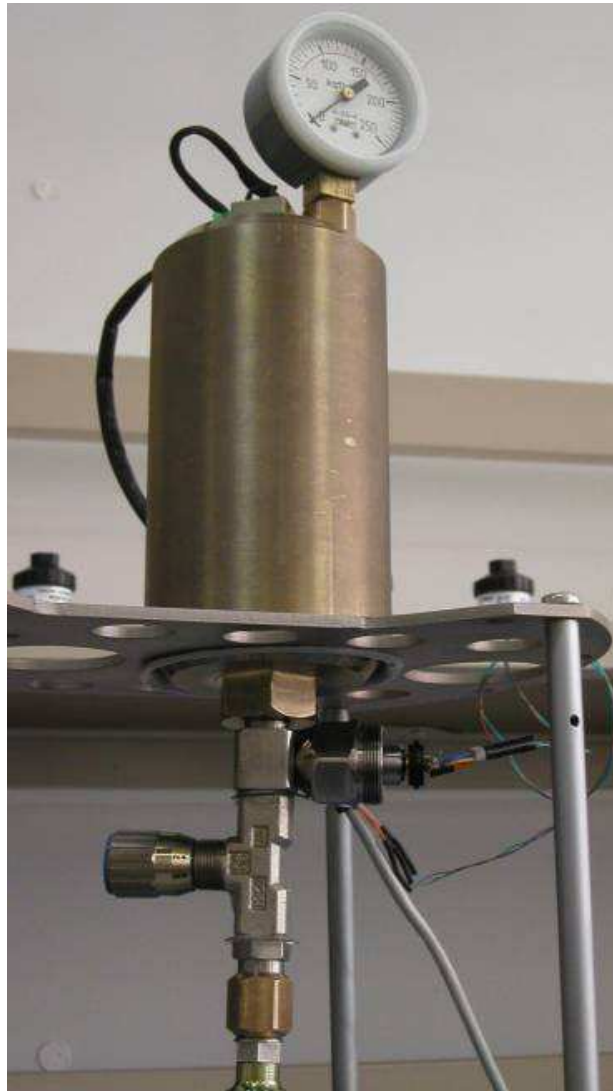
Fig 18.10-1. Test chamber showing attachment point below for pressure sensor
