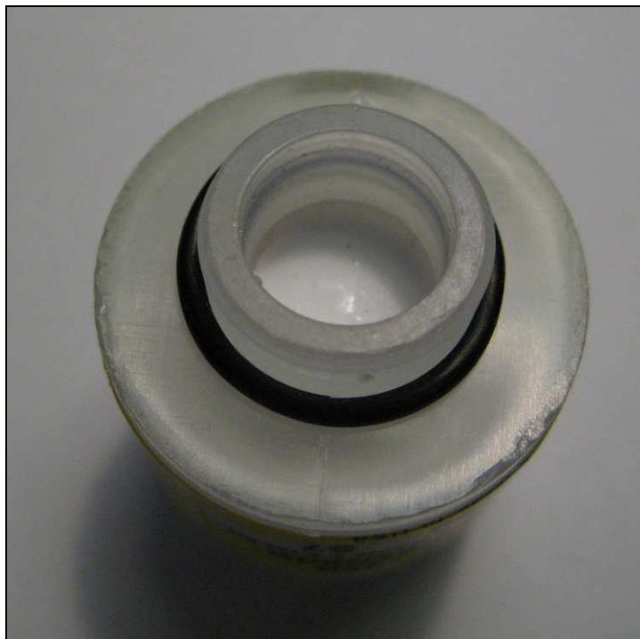
Figure 20.7-3 Electrolyte drops on the sensor membrane
