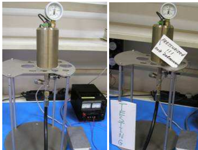
Fig 18.9-1. O2 sensor test fixture. Gauge on top of chamber is for safety only: pressure readings were taken digitally (electronically).
