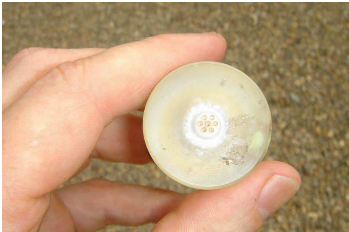
Fig 15.1-1: Front face of Insovt DK-32 showing integral and thick shield in front of hydrophobic membrane to prevent membrane lifting when depressurised rapidly. Sensor serial number 171, shown after testing.
