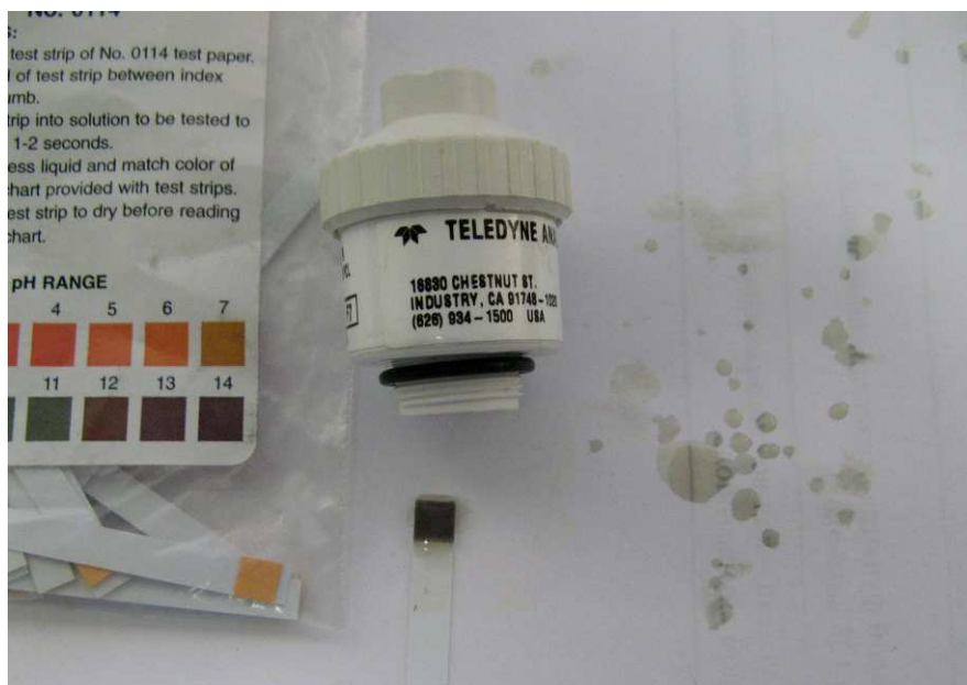
Figure 20.7-1 Electrolyte drops from Sample 2 after shaking over paper. Litmus indicator shows pH 14 when moistened with the drops. Electrolyte continued to leak after the tests, and 2 months later the sensor appeared to be dry. Equipment user manuals should warn users of the caustic risk from oxygen sensors.
