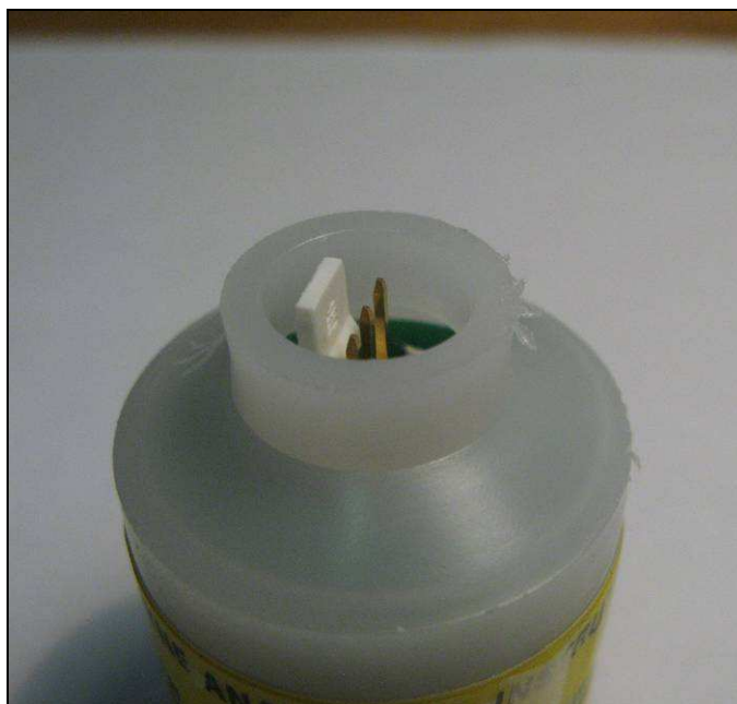
Figure 20.7-4 There is a small dent near the connector port of the sensor, but no other visibly apparent damage.
