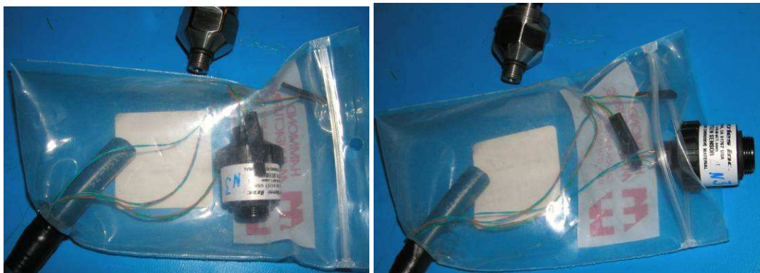
Fig 18.12-1. PPO2 sensor in/out of plastic bag with CO2 feed.
