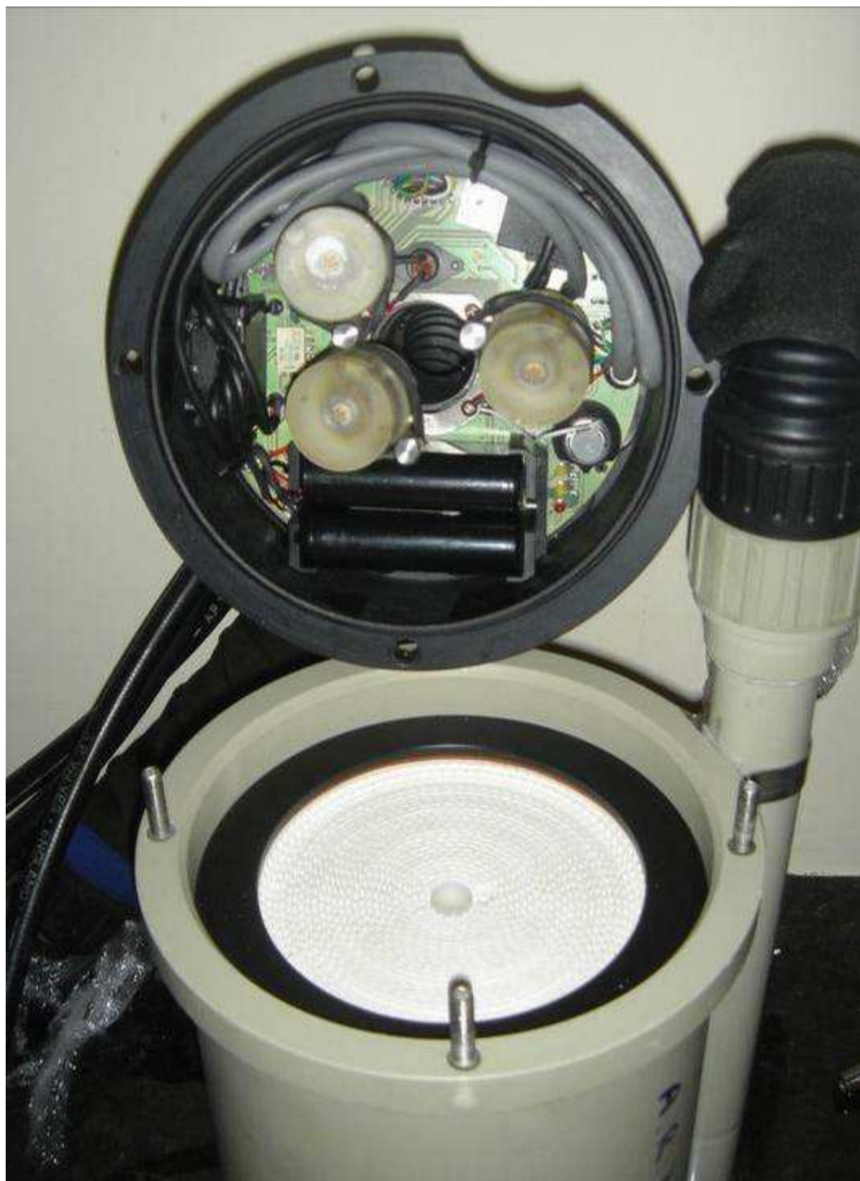
Fig 15.1-5: Test Rig using an improved AP Valves Inspiration Classic to test the Insovt DK.32s on dives. An ExtendAir scrubber was fitted, the batteries were replaced by rechargeable lithium ion cells and the failure point at the top of the lid was removed by Deep Life. Note that cells within the breathing loop are not used in any rebreather design by Deep Life, other than in this test fixture.
